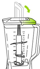
3. Align arrows on lid and handle, then lower handle to lock in place.
