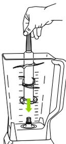
2. Holding the Stacked Blade Assembly by the top of the shaft, insert it into the pitcher.
