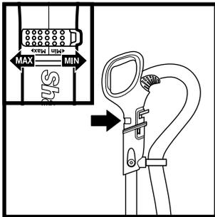
**Suction Control Collar** offers variable suction based on your needs. Slide to **MIN** to reduce suction and increase maneuverability on carpets. Slide to **MAX** to increase suction on bare floors.
