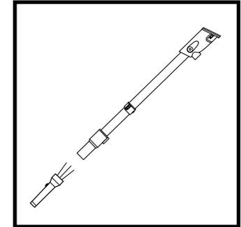
Detach wand from floor nozzle and handle, and check both ends for blockages.
