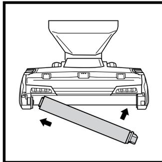
To remove the **Soft Roller** from the nozzle, lift it out by the pull tab and tap off any loose debris. Use a dry towel to wipe the Soft Roller clean, or to remove any debris caught in the teeth behind it.
