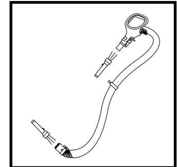
Detach handle from wand and hose from the vacuum pod, and check openings for blockages.
