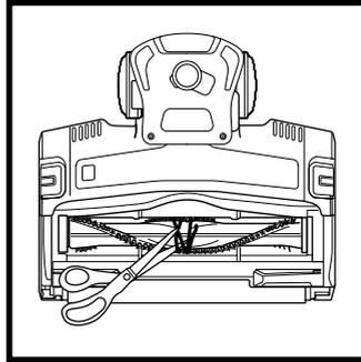
To open the brushroll garage, slide both release buttons on the floor nozzle away from you, toward the back of the nozzle, then lift off the lid. Clear away any objects or debris.
