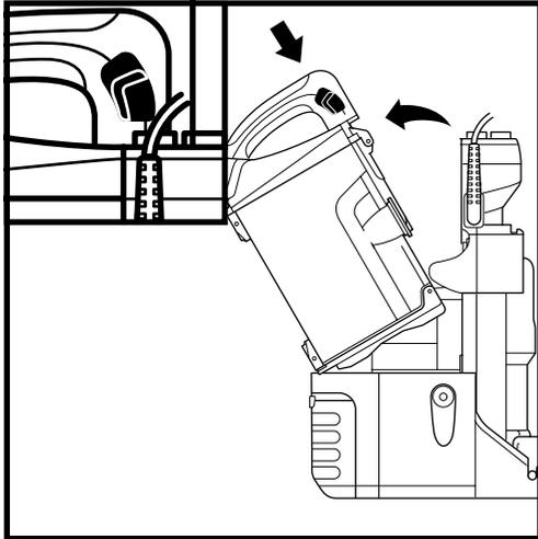
To remove **Dust Cup**, slide up the buttons on both sides of the handle. Tilt dust cup, then lift to remove.
