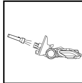
Detach wand from floor nozzle, tilt nozzle neck back, and check opening for blockages.
