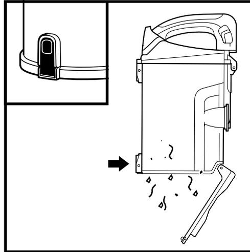
To empty debris, press lower release button and bottom of dust cup will drop open.
